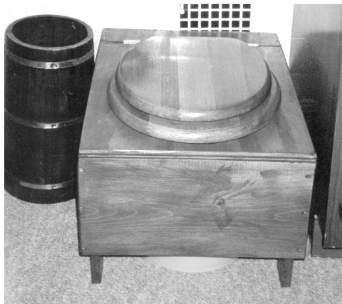
9. Attach your seat. Stain, varnish or paint the wood. You now have a compost toilet!
