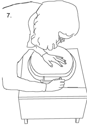
7. Mark holes for toilet seat attachment.
